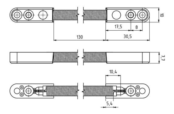
Please leave a cable loop. This will ensure that adequate cable is available for sliding on opening the door.
